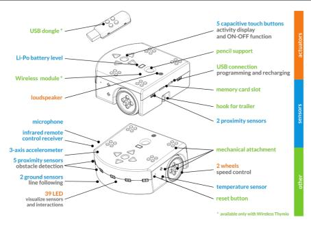
To turn Thymio on, touch the round button that lies in the center of the four arrow buttons until the robot makes a sound and turns green. It takes just a few seconds.
